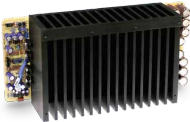
The heart of the Nº 500H Series amplifiers – elegant simplicity. The use of multiple smaller capacitors allows them to be physically closer to the amplifiers themselves providing for greater transient response when power is needed immediately. The Nº 531H, Nº 532H and Nº 533H each have sixteen output transistors per channel while the Nº 535H has twelve per channel. All models are fully-differential designs with robust power supplies and are stable into 2 ohms.
